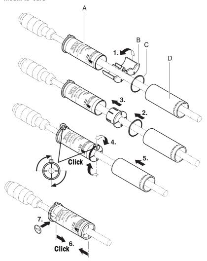
1. Check whether the measuring data sticker for the set weighing platform configuration and, if necessary, also the EC calibration symbol (green M), has (have) been applied to the inner socket (A) of the ID card.
